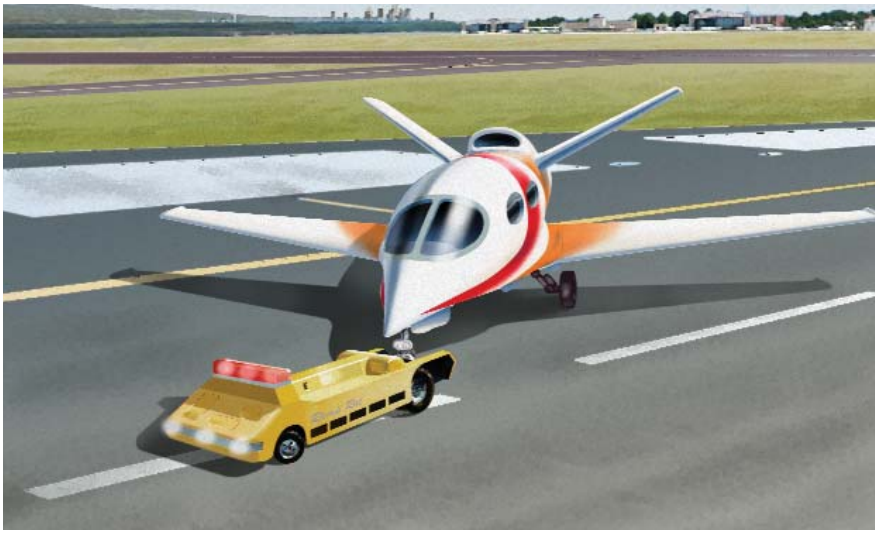
Future FBO ground handling movements will be conducted through the use of low-slung, computer-controlled tugs such as the Ramp Rat. These automated tugs may help to eliminate aircraft damage caused by hangar rash and towing accidents.
